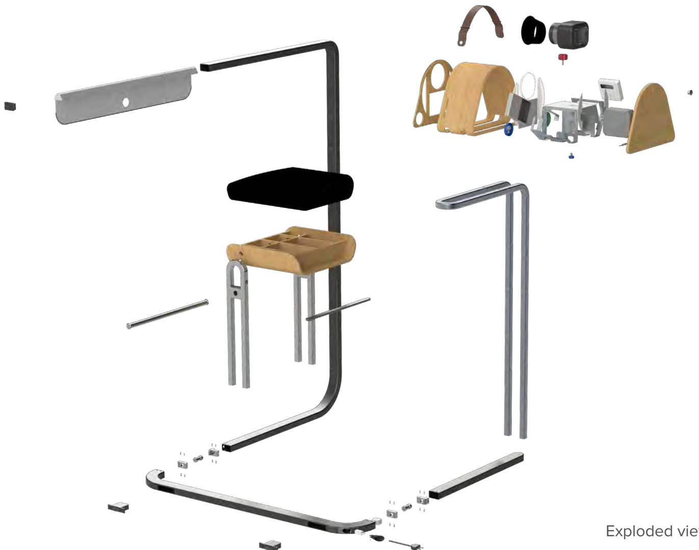
Easy assembly using sheet metal part
